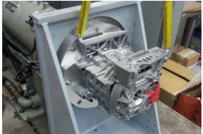
Mounting a motor and inverter to a precision dynamometer
