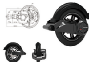
H45 Side mounted motor H45侧挂电机
